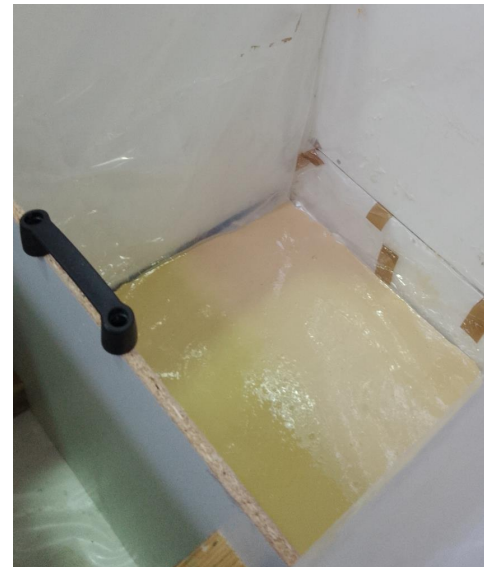
casting and foam growth
